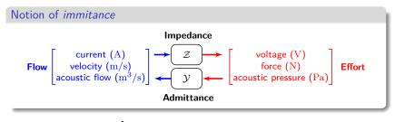
Linear system:  $Y(s) = \frac{1}{Z(s)}$  (with s the Laplace variable)
