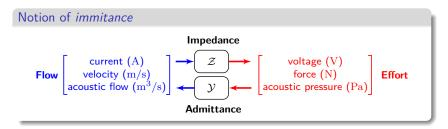
Linear system:  $Y(s) = \frac{1}{Z(s)}$  (with s the Laplace variable)
